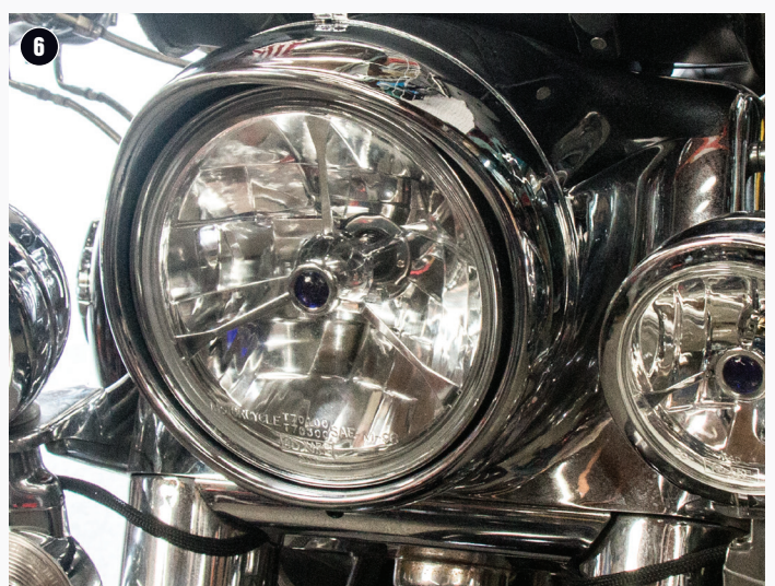
3. The new LED headlight bulb fits into the bike's stock headlight lens assembly. It is retained in the same manner as the stock headlight bulb.
