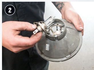
3. The new LED headlight bulb fits into the bike's stock headlight lens assembly. It is retained in the same manner as the stock headlight bulb.
